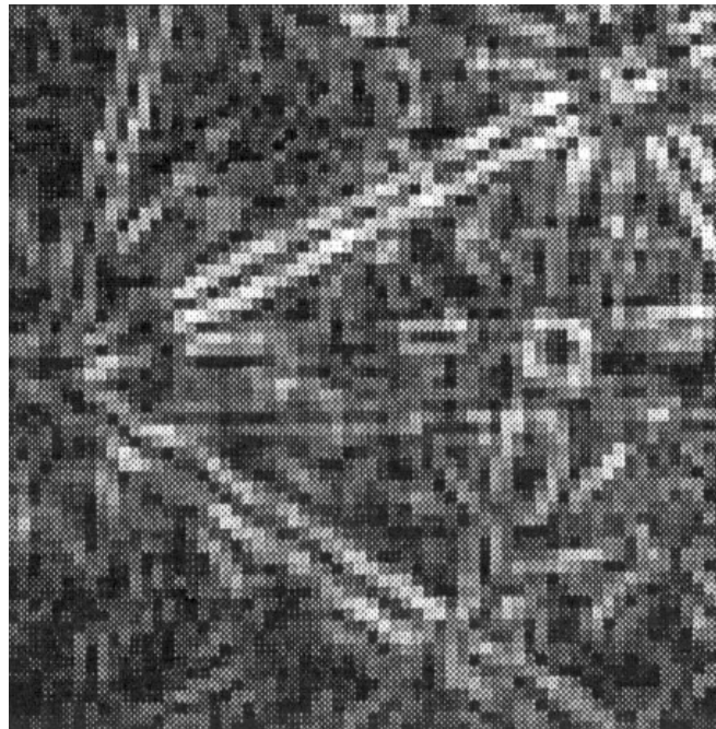
Figure 4.1.2 The gradient magnitude of the image in figure 4.1.1, based on the 3x3 Sobel operators.
